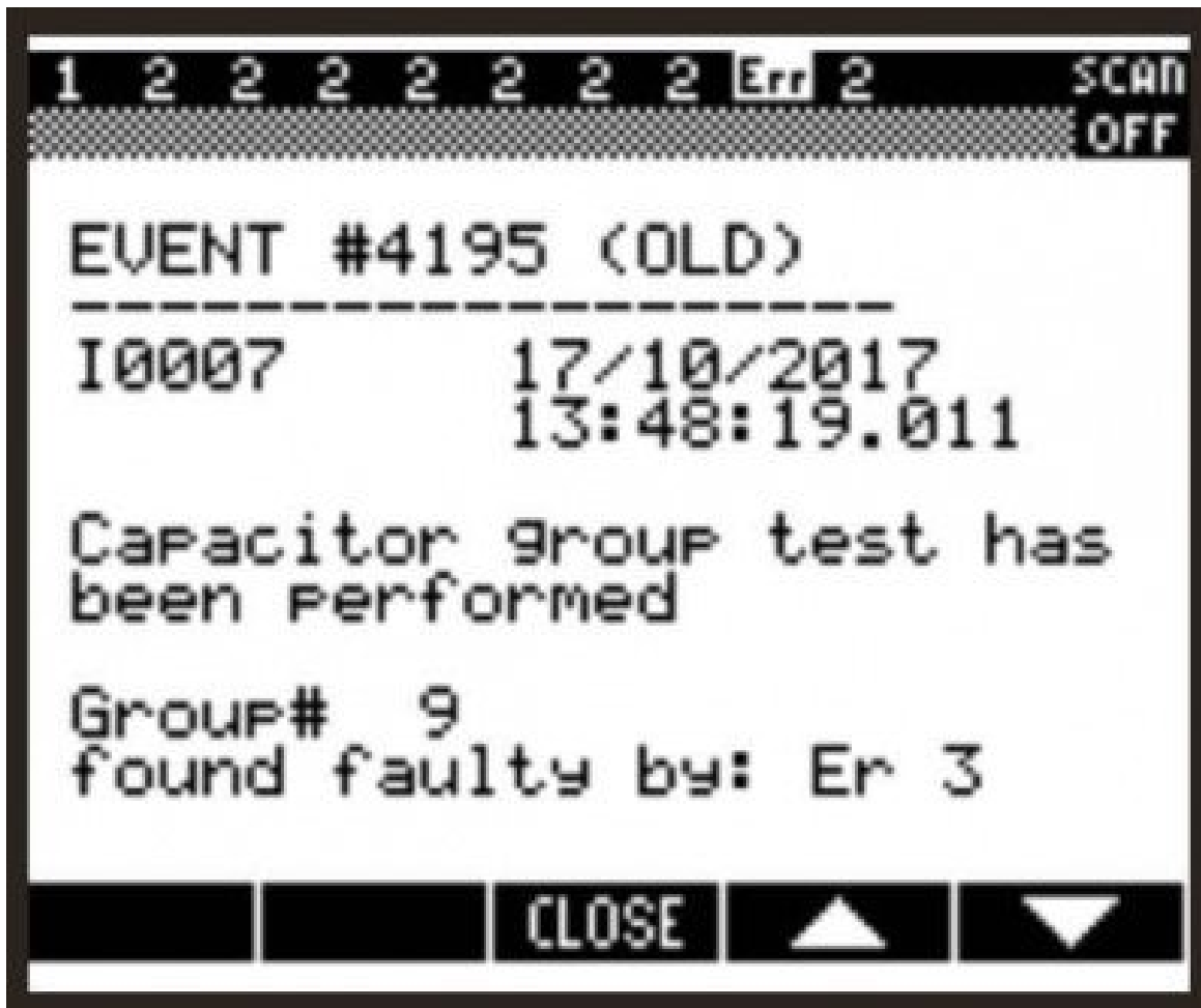
Figure 3: Controller fault screen
