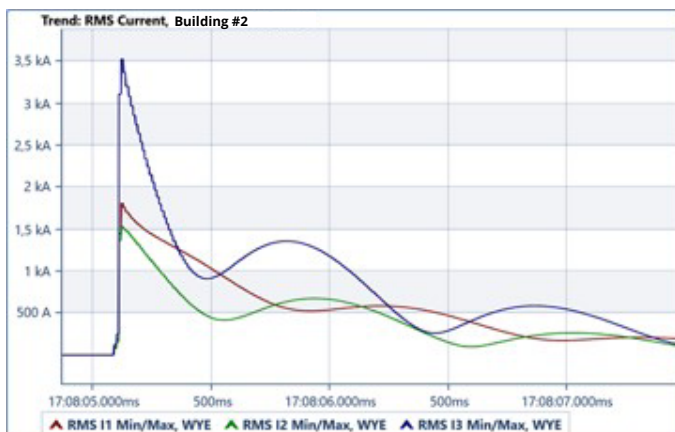
MV side Power Quality recordings – Building #2 MV transformer inrush
